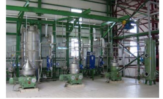
Refining process is applied with the aim of giving the oil edible properties by removing the non-oil impurities from the oil in a way that causes the least damage to the triglyceride structure of the oil and tocopherols. In general, raw oil contains free fatty acids (FFA), gum (phospholipids), peroxide and oxidation products, metals and unsaponifiables, in addition to triglycerin.
